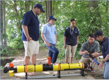
USNA Oceanography Department faculty engage in AUV training prior to deployment. Shown is the i3XO EcoMapper from Xylem's YSI Integrated Systems and Services. Built on the Iver3 platform from OceanServer Technology, the i3XO is the newest AUV to come from the 10-year-old partnership between the two companies.
