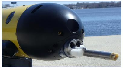
(Top and Bottom) With sonar and bathymetric surveying, overlaid with georeferencing, AUVs can provide detailed imagery of ocean, coast, lake and river bottoms. The nose of the Eco-Mapper contains object-avoidance sonar and high-resolution sondes for collecting water quality data.
